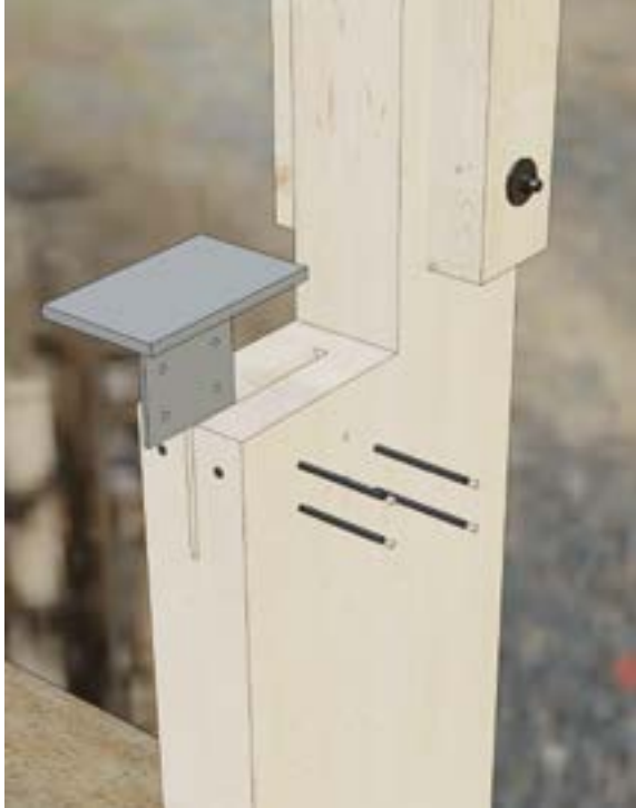
Craneway stanchion with support steel part for building site crane track.
