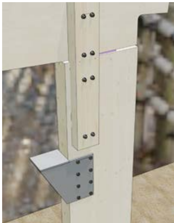
Wooden stanchion with steel craneway bracket
