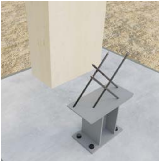
Stanchion foot with slanting screws pre-assembled on wooden support. Tabs for bracing possible. Structural tolerance compensation with millimetre plate and subsequent filling with grouting mortar possible.
