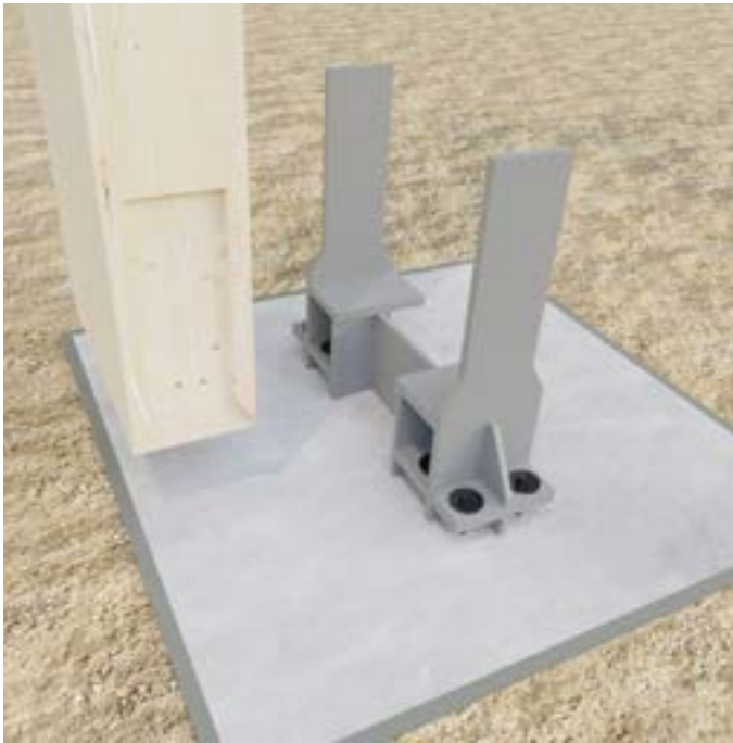
Anchor rods with thread in concrete, one-piece stanchion foot with slanting screws pre-assembled on wooden support (smaller support column widths). Wall bracing tabs possible. Structural tolerance compensation.
