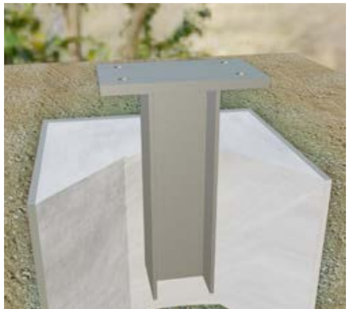
Steel foot in concrete foundation
