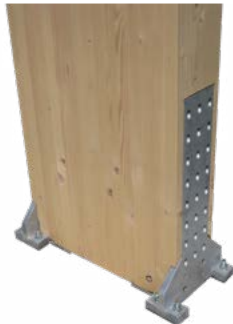
For support columns without steel plinth (interior or on concrete plinth). Connection via slanting screws, support steel part integrated in foundation with threaded rods.
