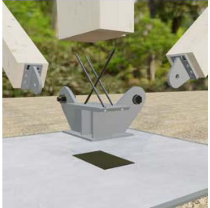
Welded base in foundation. Stanchion foot with steel plinth, with slanting screws pre-assembled on wooden support – executed here as a corner column with bracing tabs.
