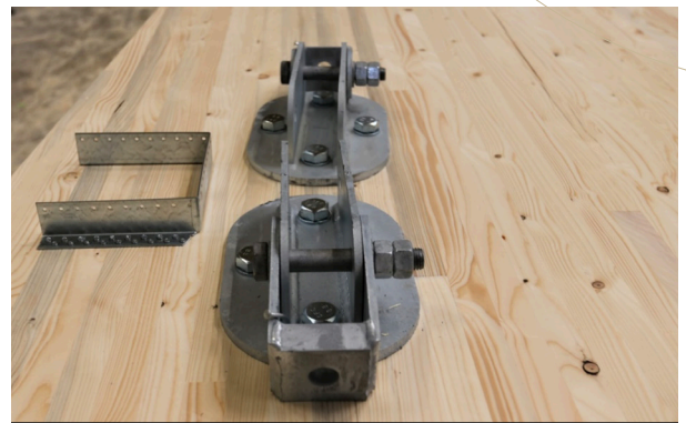
Two steel parts if the bracing inclination changes
